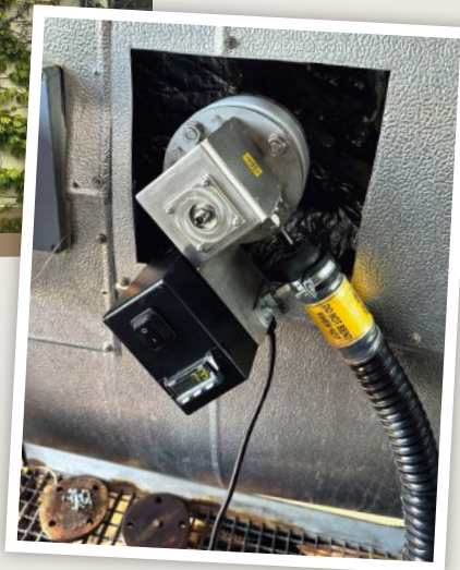
Above: Signal MCERTS approved 363SM heated pre-filter with heated line (Picture credit: Signal Group)
