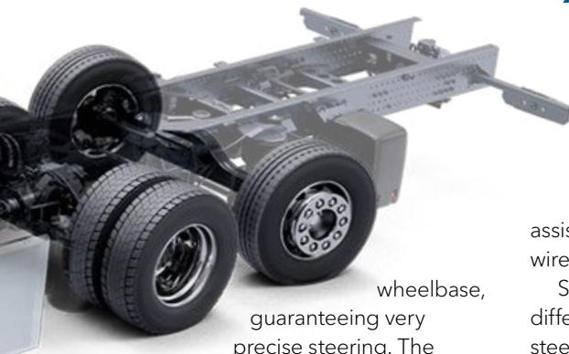
wheelbase, guaranteeing very precise steering. The turning circle of both tractor and rigid chassis models has been reduced by 12%.
